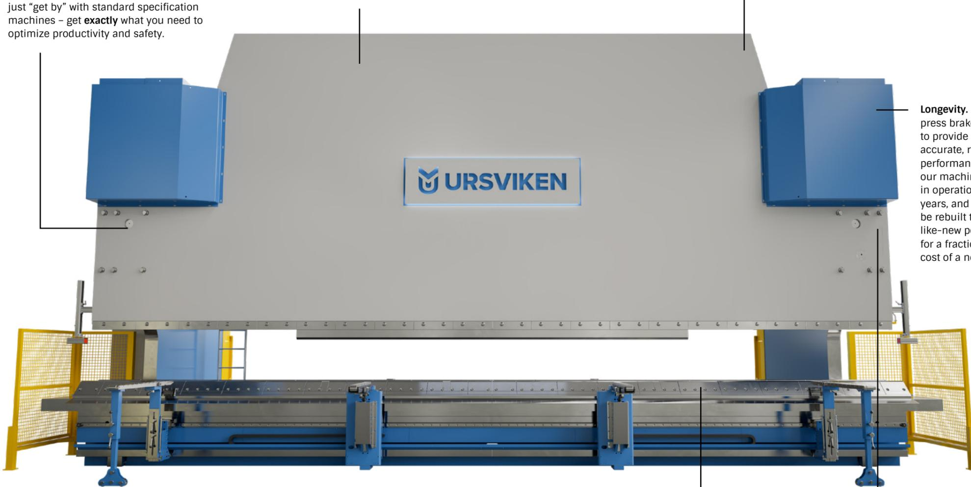
**Double Bed Reference system.** Originally invented by Ursviken in 1965, DBR is based on two independent master cylinders that automatically adjust to individually set the press beam depth, completely independent of frame deflections. DBR set a new standard of press brake accuracy that has changed the face of precision bending.
